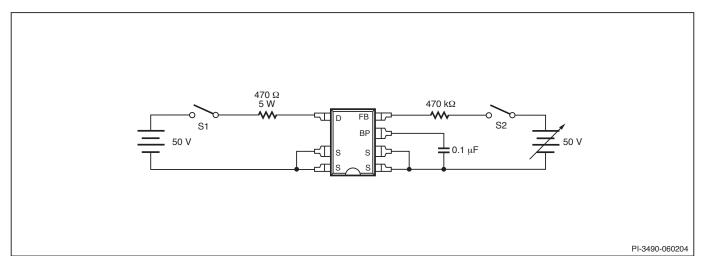
Figure 7. LinkSwitch-TN General Test Circuit.
