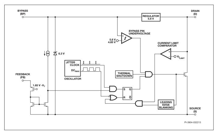
Figure 2a. Functional Block Diagram (LNK302).
