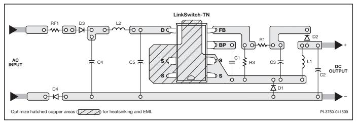
Figure 6a. Recommended Printed Circuit Layout for LinkSwitch-TN in a Buck Converter Configuration using P or G Package.
