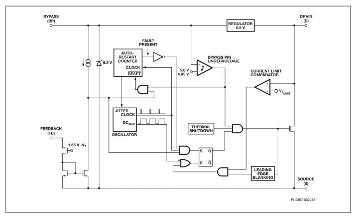
Figure 2b. Functional Block Diagram (LNK304-306).
