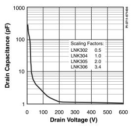
Figure 16.  $C_{\rm oss}$  vs. Drain Voltage.
