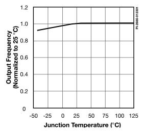
Figure 11. Frequency vs. Temperature.
