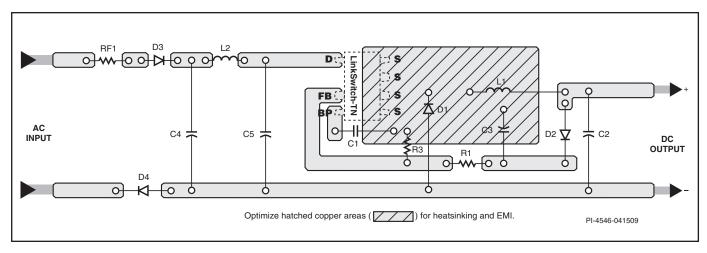
Figure 6b. Recommended Printed Circuit Layout for LinkSwitch-TN in a Buck Converter Configuration using D Package to Bottom Side of the Board.
