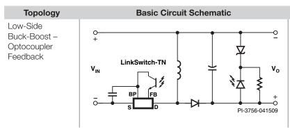
Table 2 (cont). Common Circuit Configurations Using LinkSwitch-TN.
