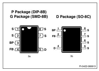
Figure 3. Pin Configuration.
