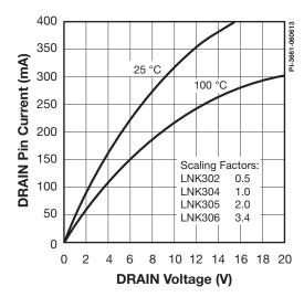
Figure 15. Output Characteristics.
