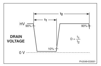
Figure 8. LinkSwitch-TN Duty Cycle Measurement.
