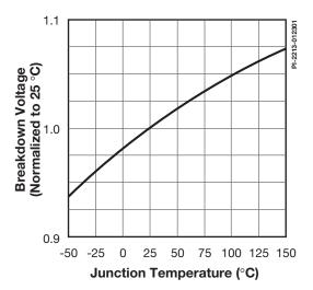
Figure 10. Breakdown vs. Temperature.
