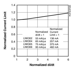
Figure 13. Current Limit vs. di/dt.
