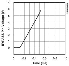
Figure 14. BYPASS Pin Start-up Waveform.
