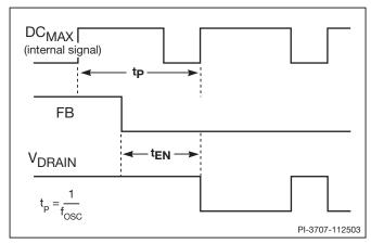
Figure 9. LinkSwitch-TN Output Enable Timing.
