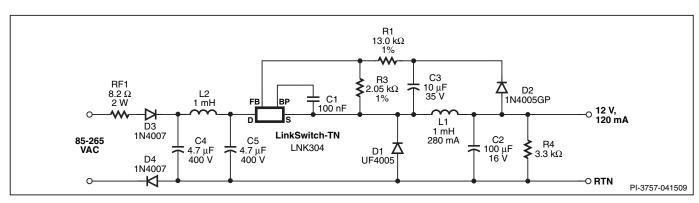
Universal Input, 12 V, 120 mA Constant Voltage Power Supply Using LinkSwitch-TN.
